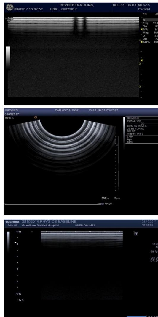
**Figure 2.** An in-air reverberation ultrasound images from different vendors.
